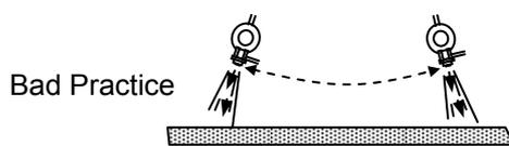
Swinging spray assembly in an arc produces poor quality material and excessive over-spray
