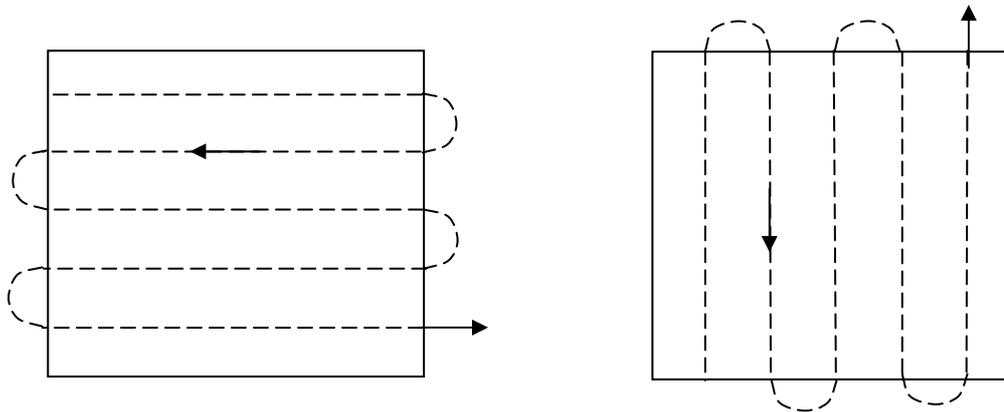
The cone shaped spray forms a strip of GRC on the mould. The next cone strip in reverse direction should overlap the preceding spray strip by up to 50%. Spraying should continue in this fashion. A well sprayed unit should not show any discrete lines of cement or glass.
