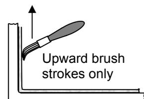
On vertical sections the brushing action should be upward only.
