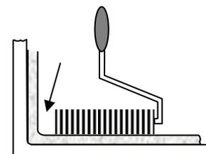
If the material has to be compacted into a corner, it is good practice to use an angled tool or a brush to press the material into the corner.
