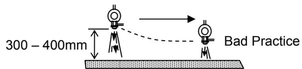
Failure to maintain constant height produces poor compaction and poor integration of layers
