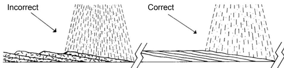
Higher cross-head speeds may be desirable when producing thin and narrow products at a high slurry output. However the inertia of the cross-head itself means that this is not always possible. Therefore, in these cases it is usually necessary to reduce slurry output and conveyor speed to achieve the same result.
